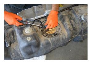
tank by turning counter-clockwise.
