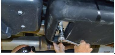
(Fig .8) Tighten the "Front Support Assembly" to specifications.
