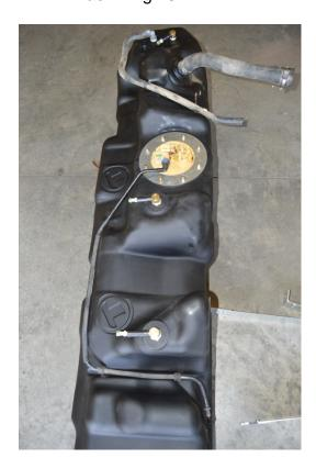
(Fig. 5) Install the hoses from the OEM tank on the new TITAN as shown above.
