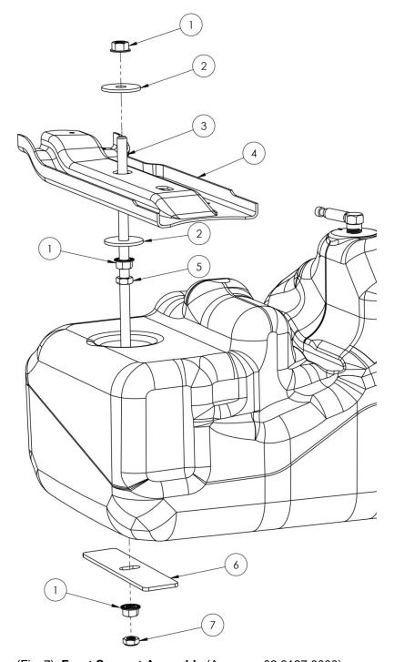
(Fig. 7) Front Support Assembly (Assy no. 03 0127 0000):
