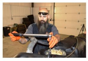
(Fig. 3) After placing the sending unit into the TITAN tank, install the top flange, and tighten the nylon lock nuts to 20 lb. ft. using a "start" pattern using a torque wrench.
