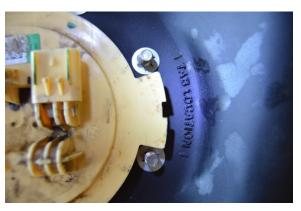
(Fig.1) Loosen the hold-down ring on the OEM (Fig.2) Be sure the tab on the sending unit lines up with the "TAB LOCATION" marks on the body of the TITAN tank as shown above.
